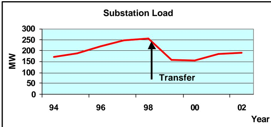
Figure 2.2.7 – Load Reduction at An Existing Substation
