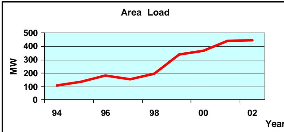
Figure 2.2.4 – Area with A Large Stainless Steel Plant Commissioned
