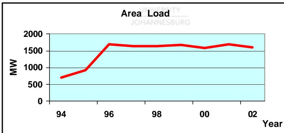
Figure 2.2.5 – Area with A Large Aluminium Plant Commissioned
