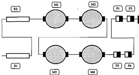
Figure 5 : Traction power circuit for series powering
