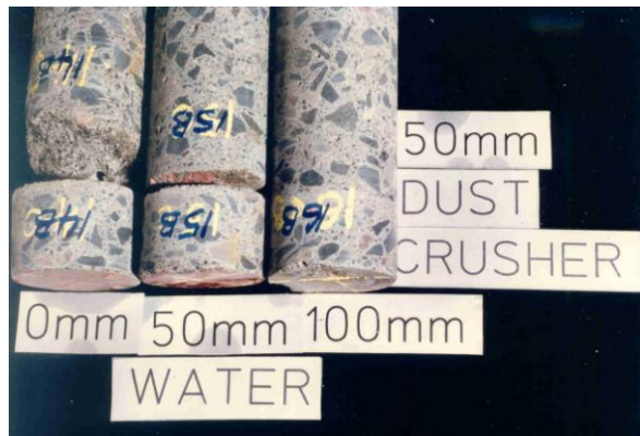
Figure 7. Close up of contact between “pile” concrete and blinding concrete for piles cast with a 50 mm layer of crusher dust at the bottom of the pile hole
