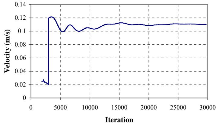
**Figure 3:** Variation of velocity with iteration (Monitoring Point)
