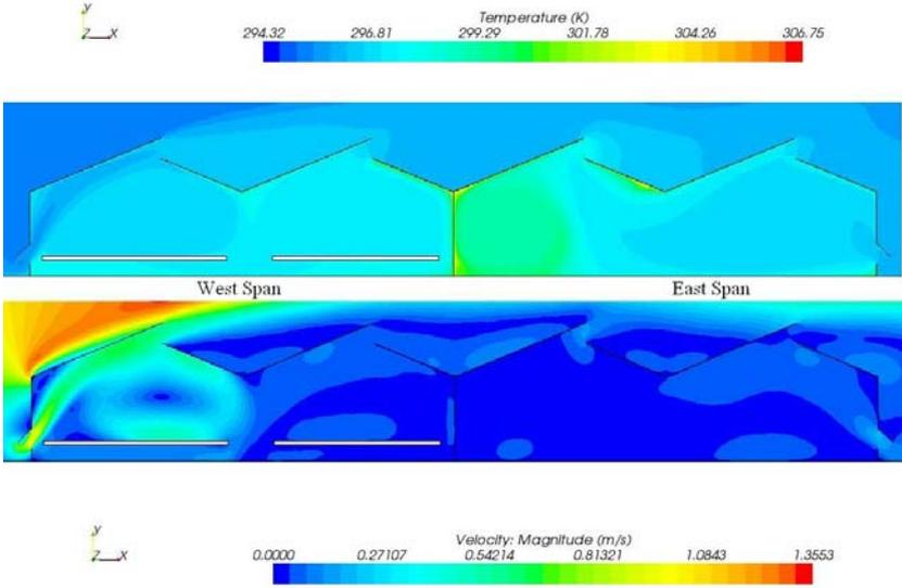
**Figure 5:** Velocity and Temperature Contour Plot (Side Vents 45°, Roof Vents Open Leeward)
