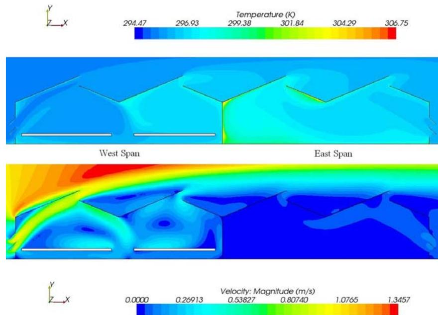
**Figure 6:** *Velocity and Temperature Contour Plots (Double Side Vents 45°, Roof vents open Leeward)*
