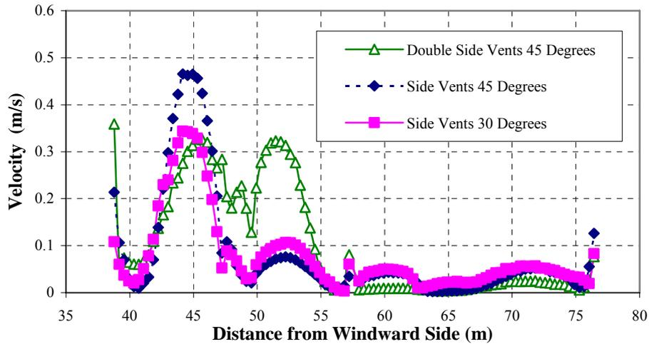
**Figure 7:** Comparison of Velocities inside Greenhouse (Roof Vents open Leeward)
