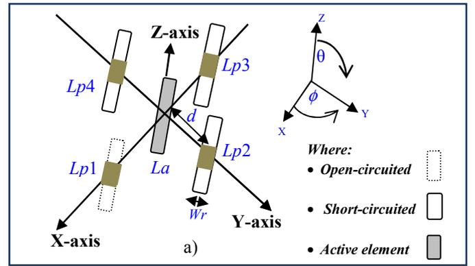
Fig. 1: Modelled antenna geometry with 5-Elements: 4 parasitic elements encircling 1 central active element.
