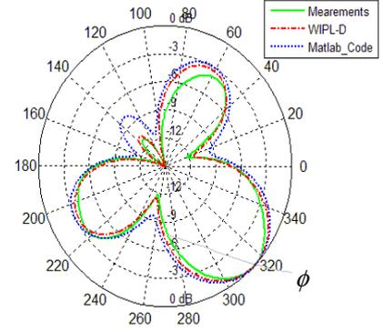
Fig. 4: Azimuth patterns for a configuration two isolated neighboring parasitic elements at  $0^\circ$  and  $270^\circ$  and two short-circuited parasitic elements at  $90^\circ$  and  $180^\circ$ ; (2N-OC).
