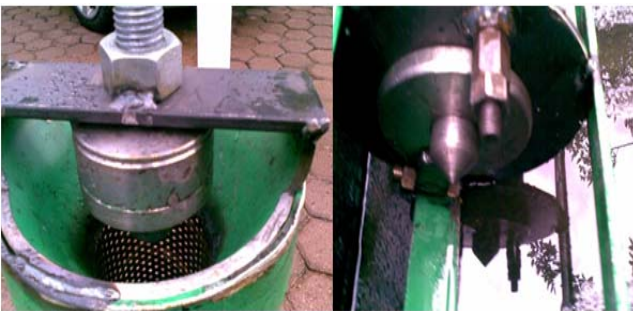
Fig. 2 Screw press equipment used for making fuel briquettes.
