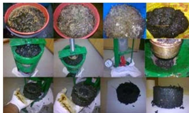
Fig. 1 Production of briquettes using a manually operated screw press
