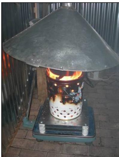
Figure 2. A typical *imbaula* on a test rig
