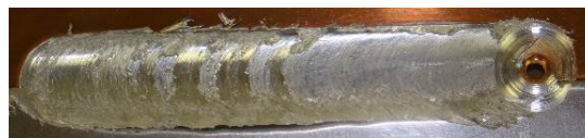
Fig. 2: Friction stir weld of aluminium and copper produced at 600 rpm and 150 mm/min
