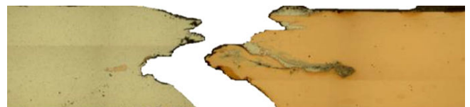
Fig. 3 (b) Fractured surface of weld produced at 1200 rpm and 300 mm/min with the 25 mm shoulder diameter tool
