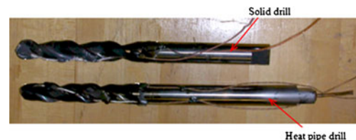
Fig. 4 Solid drill and heat pipe drill
