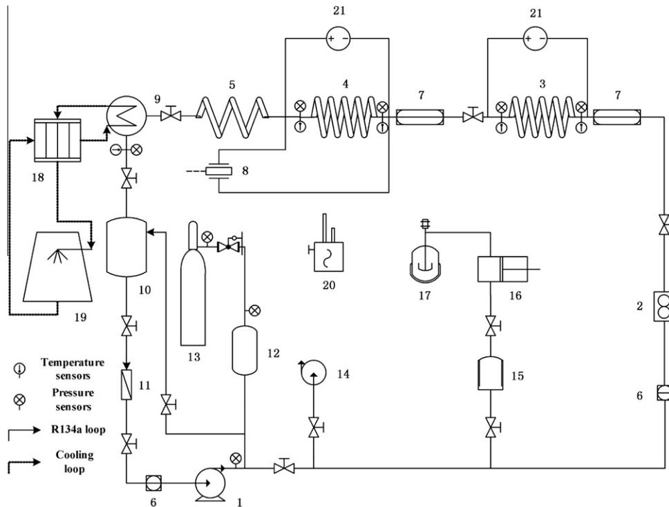
**Fig. 1.** Schematic diagram of the experimental circle loop. 1 motor pump, 2 Coriolis mass flow-meter, 3 preheating Section, 4 test Section, 5 flow pattern observing Section, 6 sight glass, 7 visual section, 8 differential pressure gage, 9 condenser, 10 receiver tank, 11 dry-strainer, 12 accumulator, 13 N<sub>2</sub> gas tank, 14 vacuum pump, 15 buffer tank, 16 refrigerant pump, 17 refrigerant tank, 18 chilling unit, 19 cooling tower, 20 halogens leak detector, 21 DC power supply.
