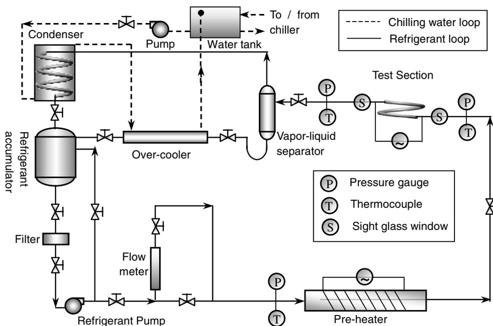
Fig. 1. Schematic diagram of the test loop.
