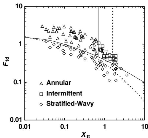
Fig. 4. Taitel–Dukler flow map for the experimental data.
