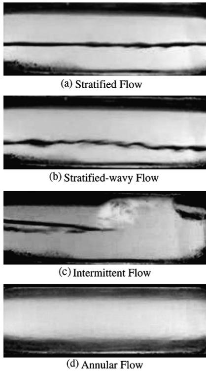
Fig. 3. Flow patterns in microfinned helically coiled tube.
