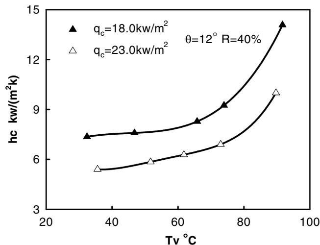
Fig. 4. Condensation heat transfer coefficient vs. working temperature.
