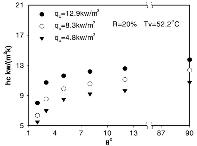
Fig. 6. Condensation heat transfer coefficient vs. inclined angle.
