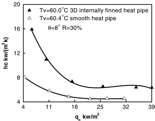
Fig. 8. Condensation heat transfer coefficient vs. heat flux.
