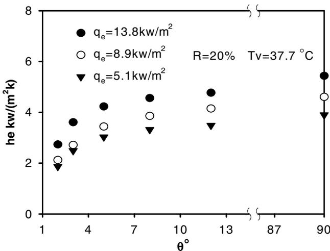
Fig. 5. Evaporation heat transfer coefficient vs. inclined angle.
