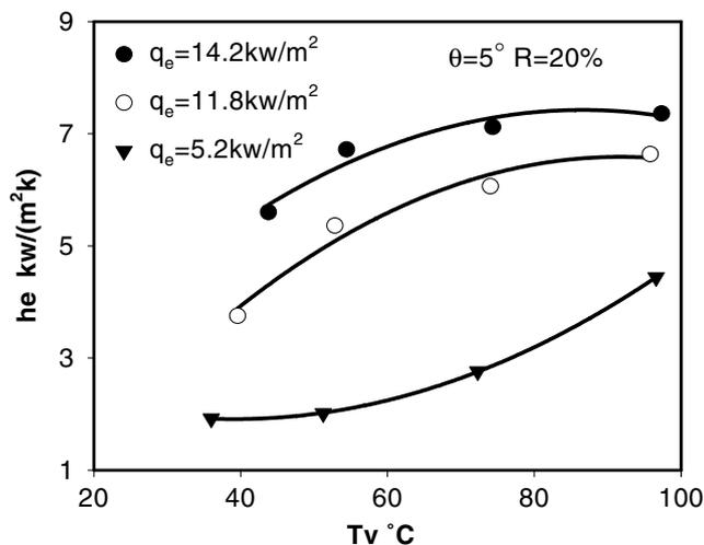
Fig. 3. Evaporation heat transfer coefficient vs. working temperature.
