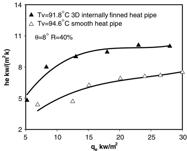
Fig. 7. Evaporation heat transfer coefficient vs. heat flux.
