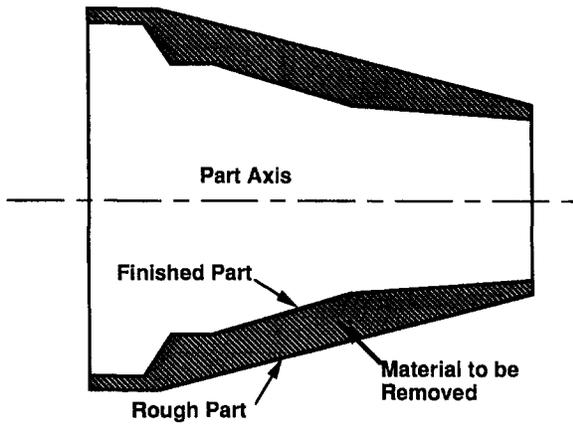
Fig. 1 Contour turning
