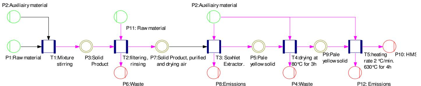
Fig.1 Flow charts for the elaboration of HMS.
