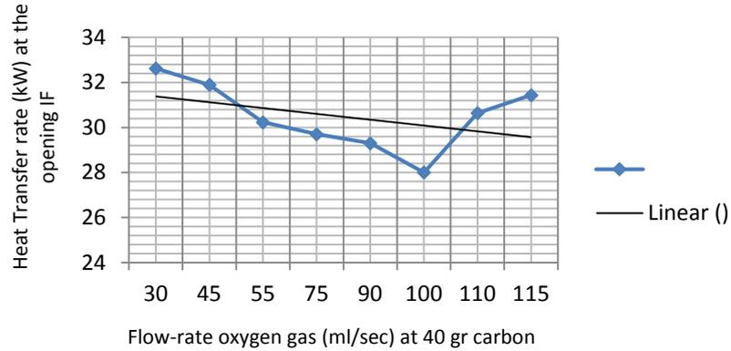
Figure 17: Comparison and variation of heat transfer at the opening due flow-rate of oxygen gas
