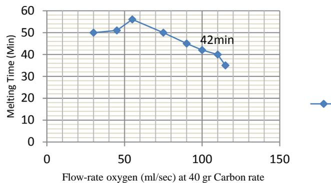
Figure 9: Variation of melting time due to Flow-rate oxygen (ml/sec) at 40 gr Carbon rate
