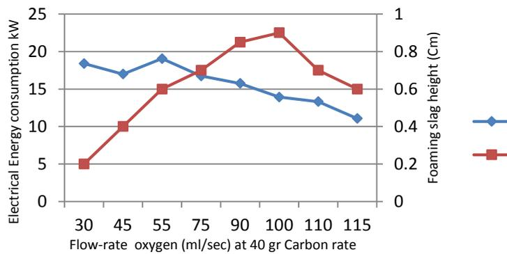
Figure 12: Relationship between electrical energy consumption (kW) and height foaming slag (cm) at flow-rate oxygen gas.
