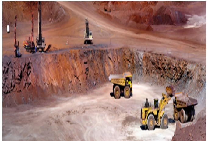
Figure 1. A mining operation of an iron ore mine, including drilling; explosion; loading; and hauling
