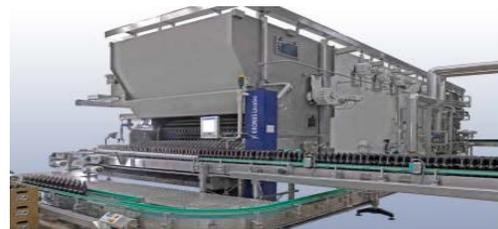
Fig 1: Bottle washer of the company under study with the gearbox
