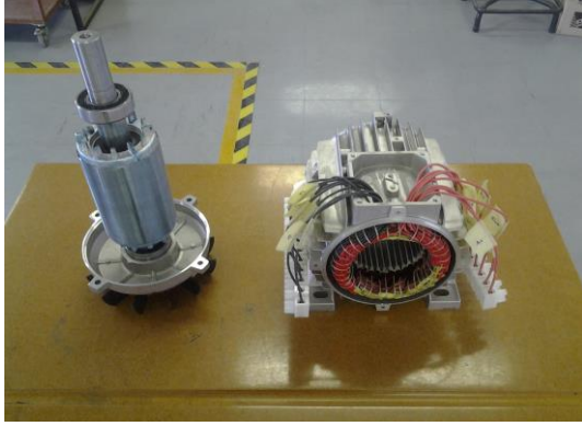
Fig. 2: Readily wound 9- phase stator (right) and squirrel cage (left)
