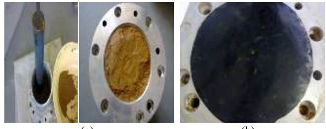
Fig. 3 (a) Soil compacted in layers (as CCL) in liner holder (b) Failed polyethylene with 5mm centred puncture overlain the CCL
