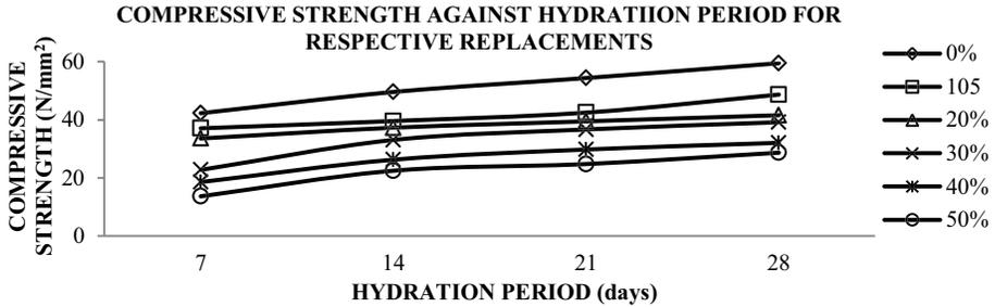
Figure 9. Compressive strength of samples with respect to hydration periods
