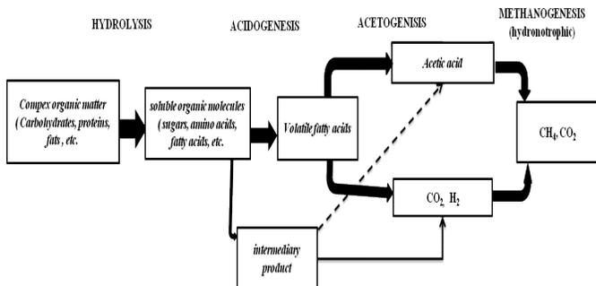
Fig. 2 Subsequent steps in anaerobic digestion of organic matter
