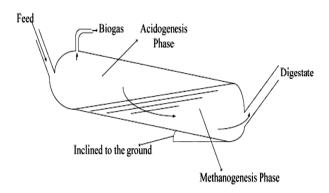
Figure 2: Schematic representation of a plug flow digester [10].
