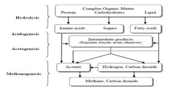
Figure 1: Anaerobic digestion pathways of organic degradable substrate [4].
