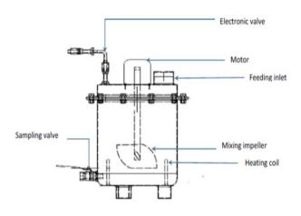
Figure 5: Schematic representation of a digester for the current study
