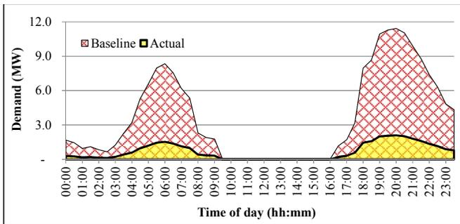
Figure 2. Incandescent and CFL demand (MW) profiles
