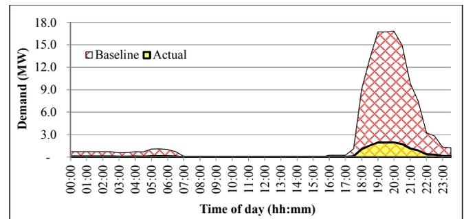
Figure 1. Downlighters and LED demand (MW) profiles
