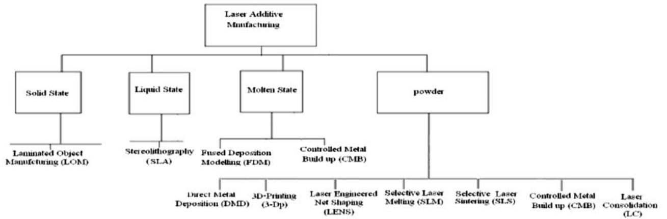
Figure 3: Classification of Laser Additive Manufacturing(LAM)
