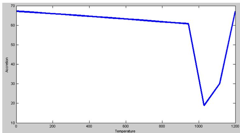
**Figure 7 Effect of temperature on ring formation**
