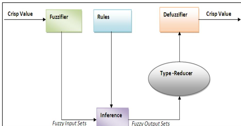
Figure 3: Type-2 fuzzy logic system (FLS)
