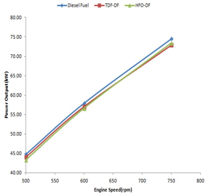
Fig. 5 Brake power output at various engine speeds
