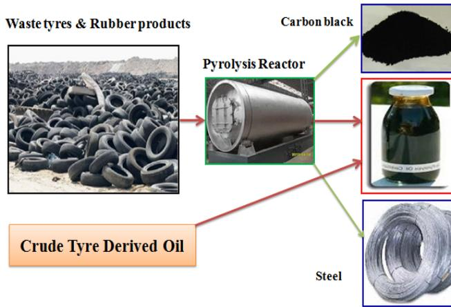
Fig. 1 Process Flow Diagram of Waste Tyre Pyrolysis
