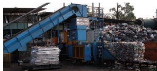
Fig. 3 Material recovery facility, paper baling machine [4]
