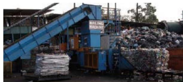
Fig. 3 Material recovery facility, paper baling machine [4]
