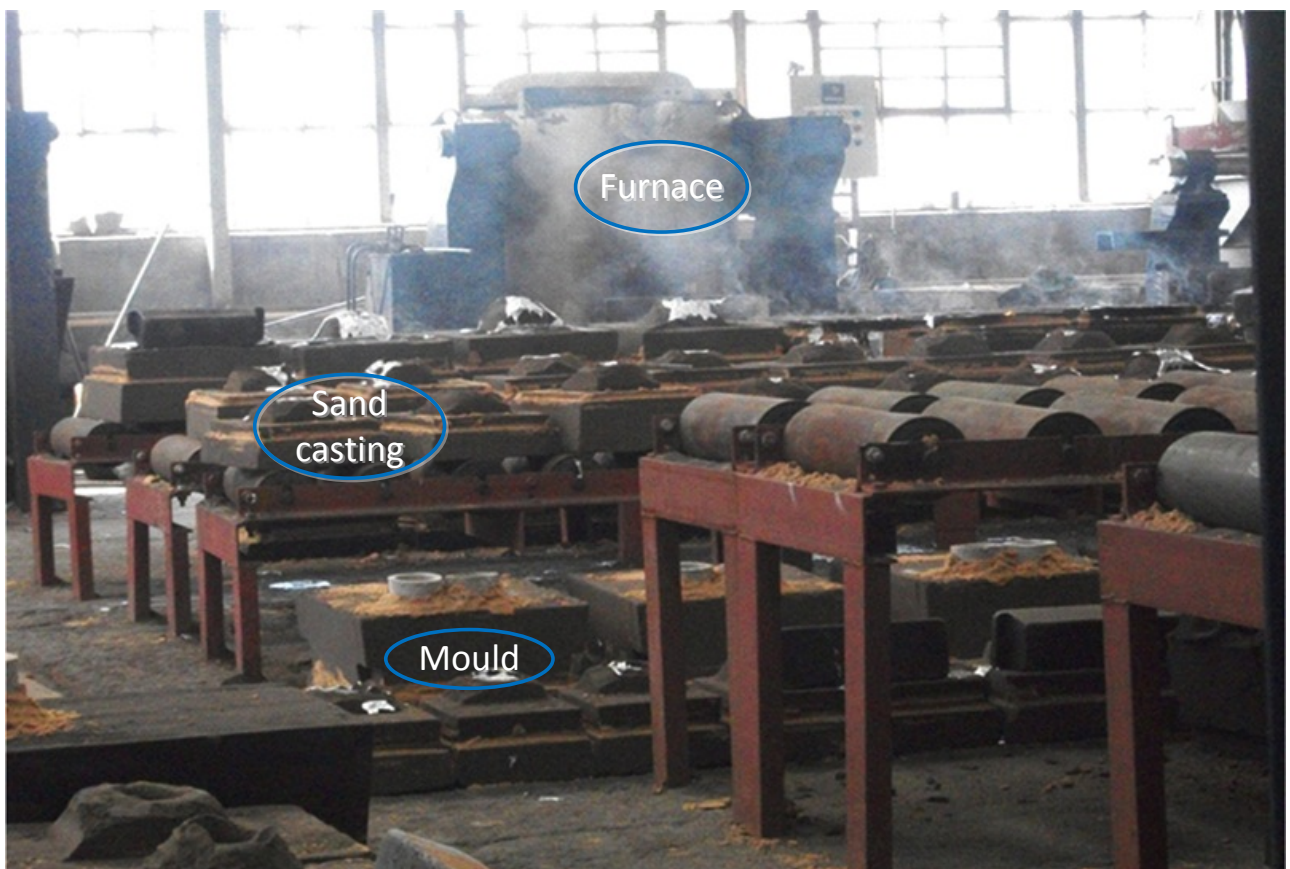
Figure 1: Sand casting plant. Source: South African foundry, 2011.
