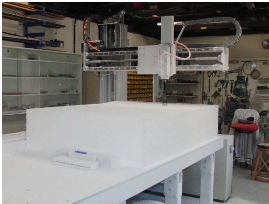
Figure 4 - CNC milling of the polystyrene plugs for the moulds of the body panels of the solar vehicle
