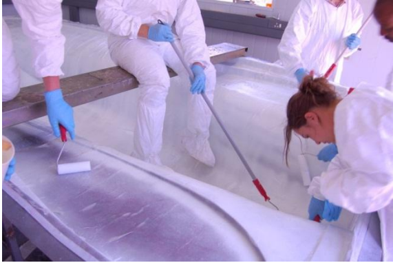
Figure 7 - Wet lay-up of composite material for final aerodynamic shell, before placed under vacuum for curing
