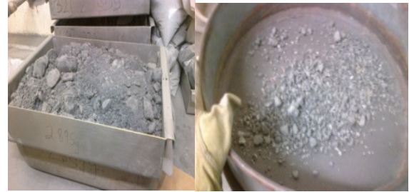
Fig. 3: Coarse screening in order to break lumps of dried samples using 600\mu m sieve
