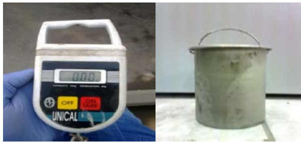
Density scale 1L Beaker Fig. 2: Pictures of sample cutter and densitometer as used in sampling campaign.
