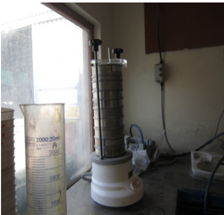
Fig. 6: Vibrating shaker used for particle size analysis
