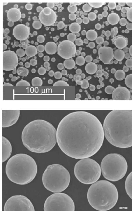
Fig.1 SEM micrographs of gas atomised powder particles
