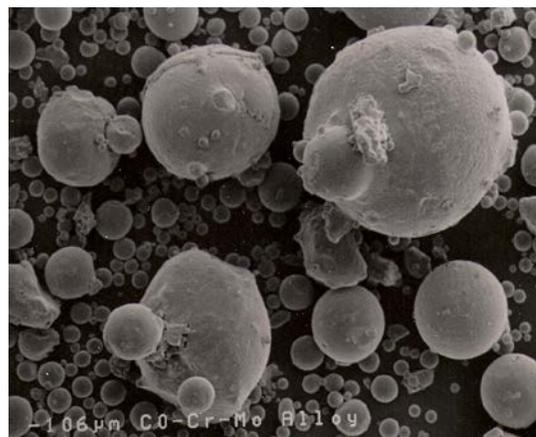
Fig. 2 Coarse Co-Cr-Mo powder with inferior surface finish
