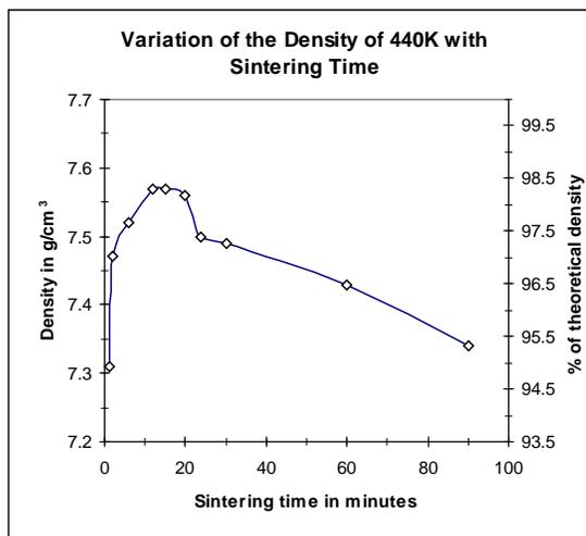
Fig. 4 Maximum density at alloy sintering temperature
