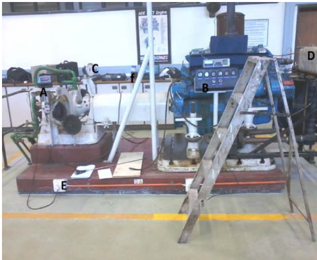
Fig. 3 Load sensor (a), start, stop, temperature sensors and fuel gauges (b), water tank (d), and sensor power input (e).
