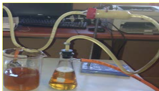
Fig. 4 Experimental set-up for single stage filtration
