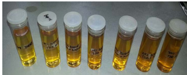
Fig. 2 Distilled pyrolysis fuel at 250°C blended with diesel
