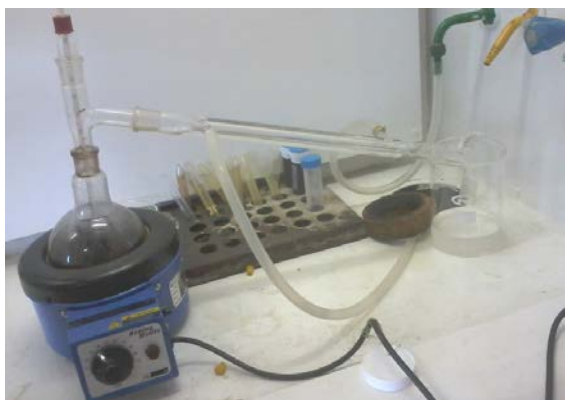
Fig. 1 Set-up for gaseous distillation of pyrolysis oil
