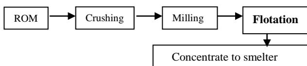
Fig. 1. Basic flow process within a concentrator
