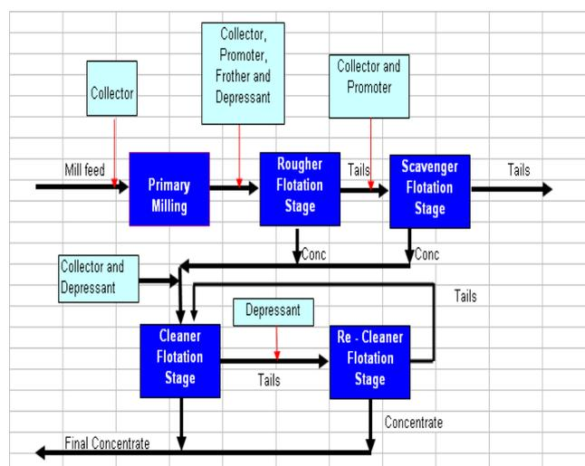
Fig. 2. Typical flow sheet of UG2 circuit
