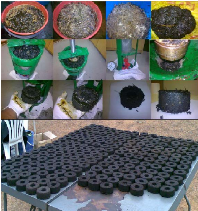
Fig. 1 Production of briquettes using a screw press
