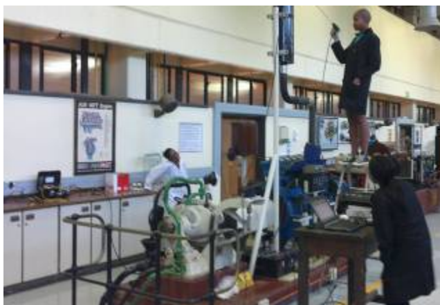
Fig. 3 ADE 407T diesel engine complete with hydraulic dynamometer and instruments, Mechanical Engineering Laboratory, University of Johannesburg
