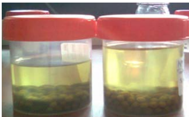
Fig. 5 Distilled rubber oil undergoing molecular filtration
