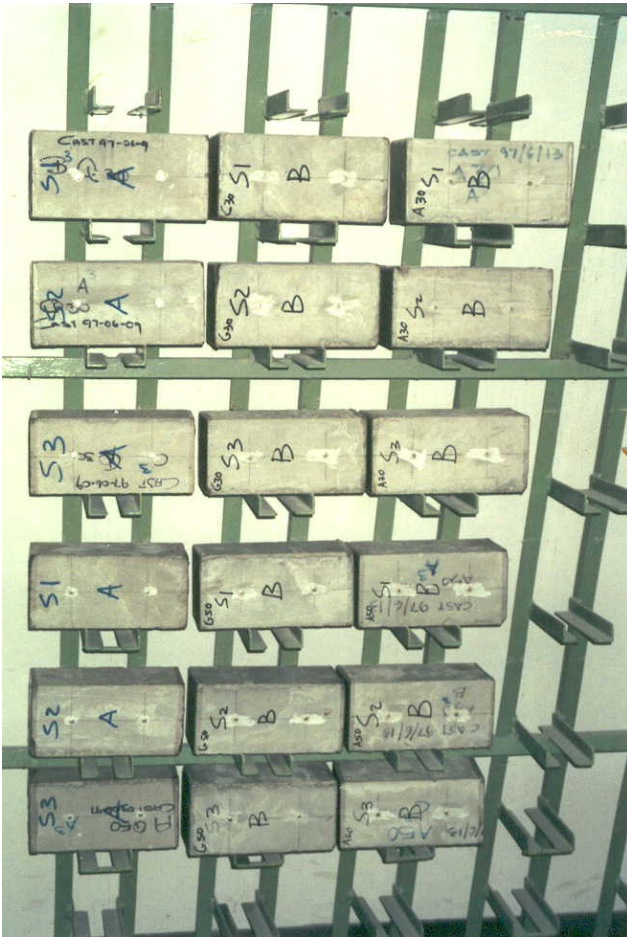
Fig.1 Drying shrinkage samples
