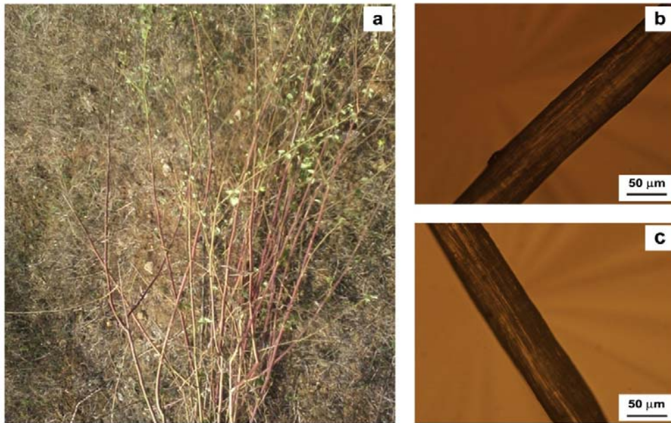
Figure 1. Photograph of (a) Thespesia Lampas plant, as well as optical micrographs of (b) untreated fiber and (c) alkali treated fiber
