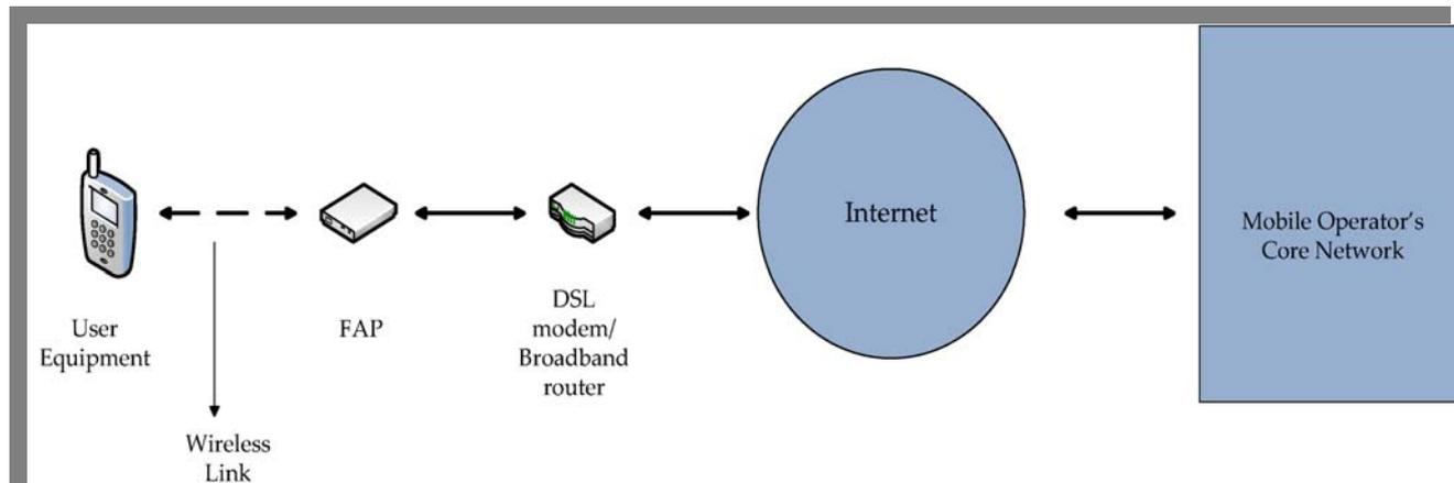
Fig 1: UE connected to an operator's core network.
