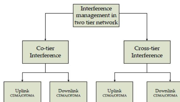
Fig 3: Types of interference in two-tier network
