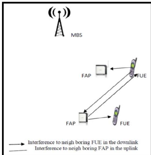
Fig 4: co tier interference between neighboring femtocells
