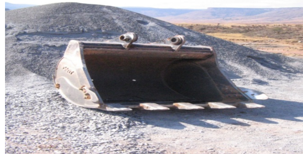
Figure 1: Worn excavator buckets for fine grained [8]
