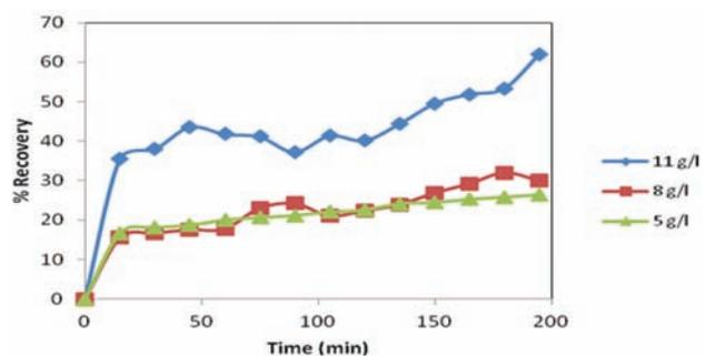
Figure 8—Percentage extraction of Ni after two-stage non-oxidative leaching with varying [Fe<sup>3+</sup>] at 90°C
