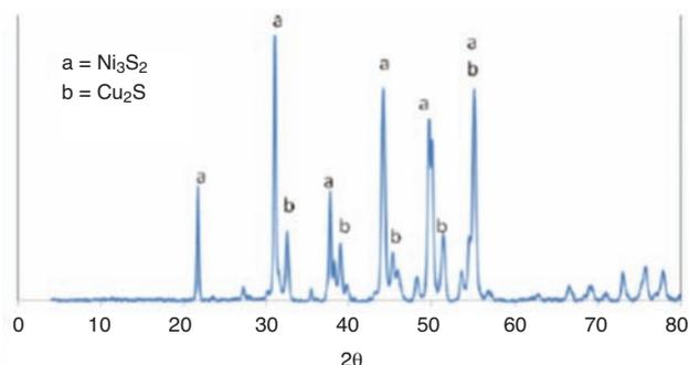
Figure 1—XRD spectra of the matte before leaching
