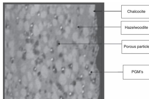
Figure 14—Electron micrograph of the matte after two-stage oxidative leaching with 11 g/L [Fe<sup>3+</sup>] at 90°C
