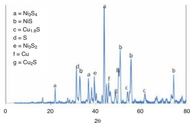
Figure 9—XRD pattern after two-stage non-oxidative leaching with 11 g/L [Fe<sup>3+</sup>] at 90°C
