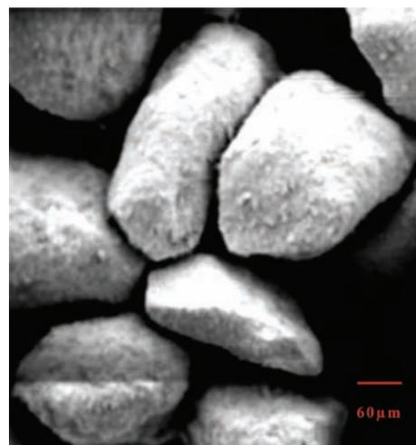
Figure 3—SEM images of the matte particle before leaching (magnification 100x)
