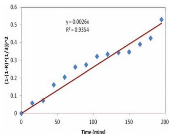
Figure 17b—Plot of the data at 90°C on the three-dimensional diffusion model by Jander
