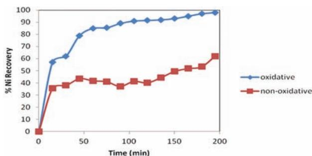
Figure 12—Ni extraction after two-stage oxidative and non-oxidative leaching with 11 g/L [Fe<sup>3+</sup>] at 90°C
