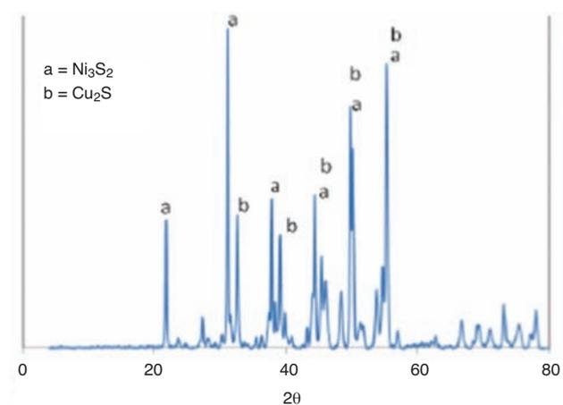
Figure 7—XRD pattern after single-stage non-oxidative leaching with 5 g/L [Fe<sup>3+</sup>] at 90°C
