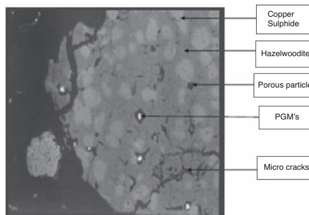
Figure 11—Electron micrograph of the matte after two-stage non-oxidative leaching with 11 g/L [Fe<sup>3+</sup>] at 90°C
