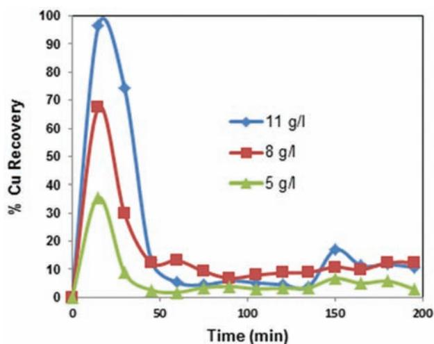
Figure 10—Percentage extraction of Cu after two-stage non-oxidative leaching with varying [Fe<sup>3+</sup>] at 90°C
