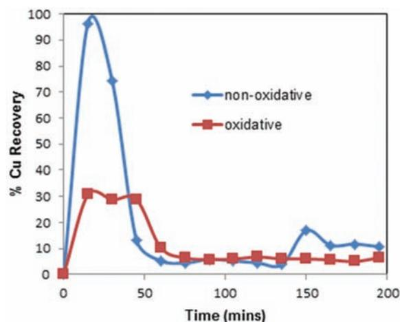
Figure 13—Cu extraction at 90°C with 11 g/L [Fe<sup>3+</sup>]
