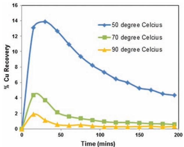
Figure 5b—Percentage extraction of Cu after single-stage non-oxidative leaching with 5 g/L [Fe<sup>3+</sup>]
