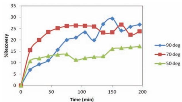
Figure 5a—Percentage extraction of Ni after single-stage non-oxidative leaching with 5 g/L [Fe<sup>3+</sup>]
