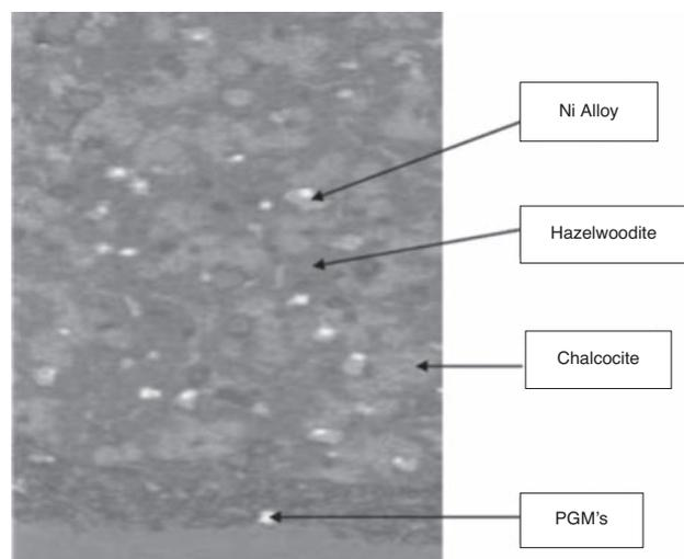
Figure 2—SEM-EDX micrographs of the matte before leaching
