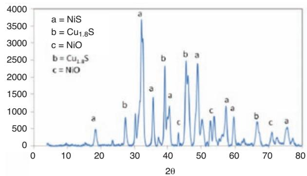
Figure 15—XRD pattern after two-stage oxidative leaching with 11 g/L [Fe<sup>3+</sup>] 90°C
