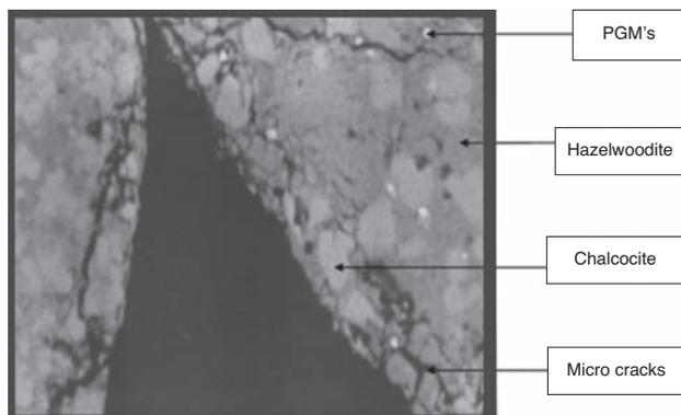
Figure 6—SEM-EDS image of the matte after single-stage non-oxidative leaching with 5 g/L [Fe<sup>3+</sup>] at 90°C
