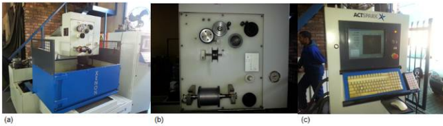
Fig. 4. (a) WEDM machine (b) wire reel (c) Actspark control console
