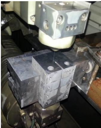
Fig. 5: WEDM of fatigue pre-crack
