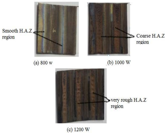
Fig. 2: The macroscopic photo of the formed samples
