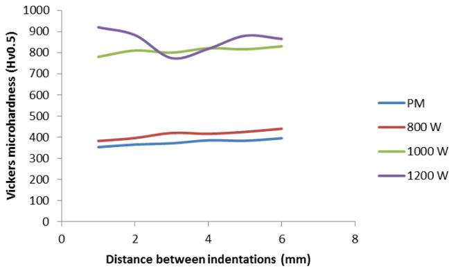
Fig. 5: Vickers hardness indentations
