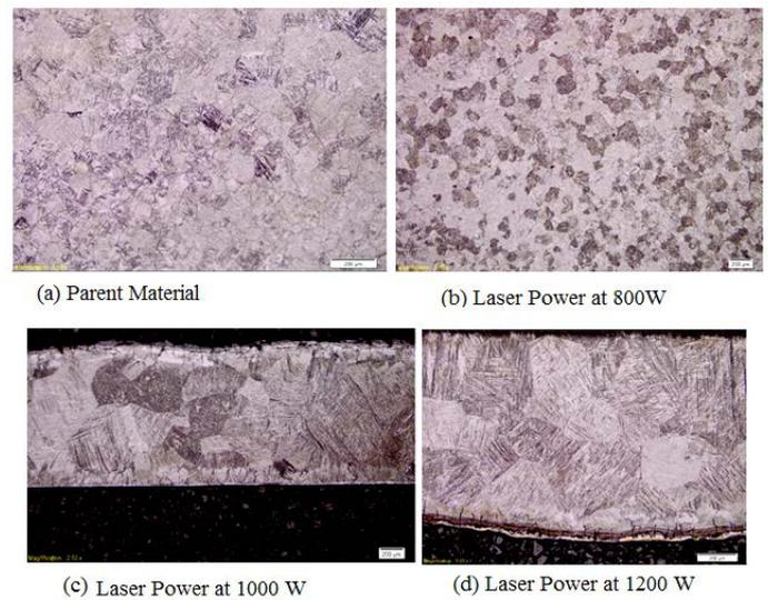
Fig. 3: Cross section of the parent material and the formed samples
