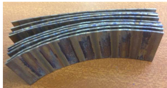
Fig. 2. Typical laser formed Ti6Al4V samples
