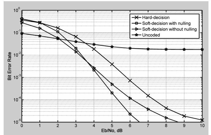
Fig. 5.  $R = 1/2$ ,  $K = 7$  and  $d_{free} = 10$  convolutional decoder bit error rate performance comparison for hard-decision and soft-decision decoding with and without nulling. Probability of NBI was set at  $P = 0.056$  and  $T$  was randomly chosen for each interference signal on a subcarrier. The NBI detection threshold was  $\gamma = 2.5\sigma_s$ . The modulation employed was BPSK and the FFT size for the OFDM system was  $N = 256$ .
