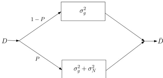
Fig. 1. Narrow-band interference model including additive white Gaussian noise (AWGN) power  $\sigma_g^2$ . At each transmission a data symbol  $D$  either enters a channel with AWGN (variance  $\sigma_g^2$ ), with probability  $1-P$ , or enters channel with noise  $\sigma_g^2 + \sigma_N^2$ , with probability  $P$ .  $\sigma_N^2$  is the variance of the NBI.
