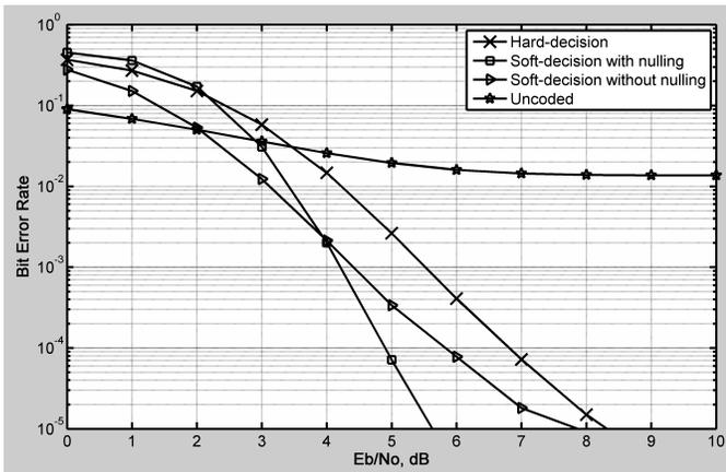
Fig. 6.  $R = 1/2$ ,  $K = 7$  and  $d_{\text{free}} = 10$  convolutional decoder bit error rate performance comparison for hard-decision and soft-decision decoding with and without nulling. Probability of NBI was set at  $P = 0.028$  and  $T = 1/100$  for each interference signal on a subcarrier. The NBI detection threshold was  $\gamma = 2.2\sigma_s$ . The modulation employed was BPSK and the FFT size for the OFDM system was  $N = 256$ .
