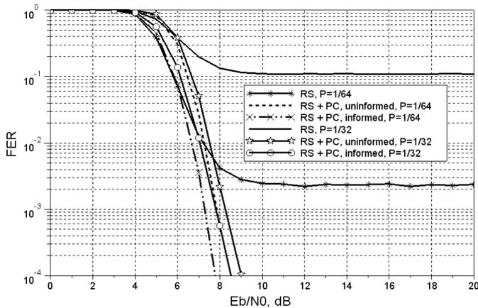
Fig. 7. Coded Scheme A, in the presence of frequency disturbances with  $T = 0.01$  and  $A = 1$ , for an informed and uninformed receiver. A (64, 48) RS only, and a concatenated (32, 24) RS code and permutation code are compared for frame error rate.
