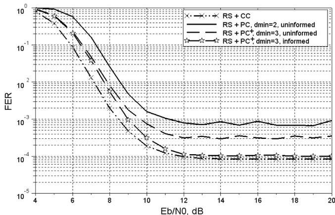
Fig. 8. A concatenation of: (32, 24) RS code and ( $M = 4, d_{\min} = 2$ ) permutation code, (32, 24) RS code and ( $M = 4, d_{\min} = 3$ ) permutation code, and (32, 24) RS code and ( $R = 1/2, K = 7, d_{\text{free}} = 10$ ) convolutional code are compared on Scheme A in the presence of frequency disturbances, for  $P = 1/16, T = 0.01$  and  $A = 1$ .
