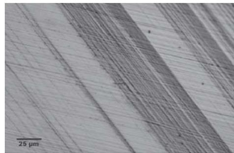
**Figure 1715: Microstructure showing Twins [22]**
