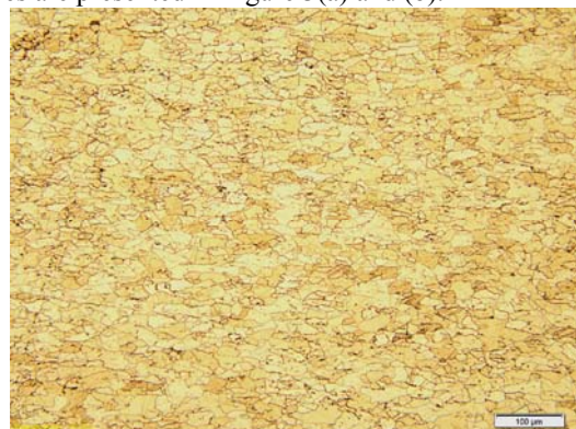
Figure 3 (a): Microstructure of the parent material
